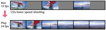
provide 2x quick-motion when standard playback
