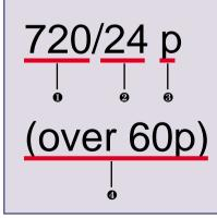
The initial numbers "720" indicate that there are 720 scanning lines per frame. The larger the number, the higher the resolution as a still image.
