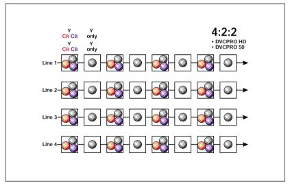
DVCPRO HD and DVCPRO 50 convert video signals to digital component signals at a 4:2:2 sampling (digitizing) ratio before recording. The resulting 4:2:2 digital component signal complies with the SMPTE259 Standard SDI signal specified in ITU-R601.
