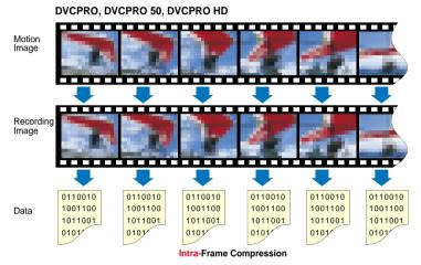
DVCPRO family: The data from each frame is compressed independently, so each frame can be reproduced singularly.
