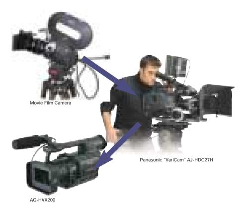
Shooting techniques called overcranking and undercranking are often used when producing movies with a film camera. They achieve unique visual effects by running the camera faster (overcranking) or slower (undercranking) than the standard playback speed of 24 fps. Playing an overcranked film at normal speed yields a slow-motion image, while an undercranked film shows the image in fast motion.
