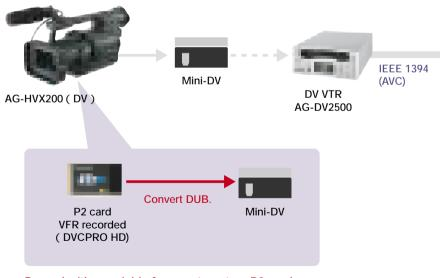
Record with a variable frame rate onto a P2 card, then dub it onto DV tape to achieve speed effects in your existing DV environment.
